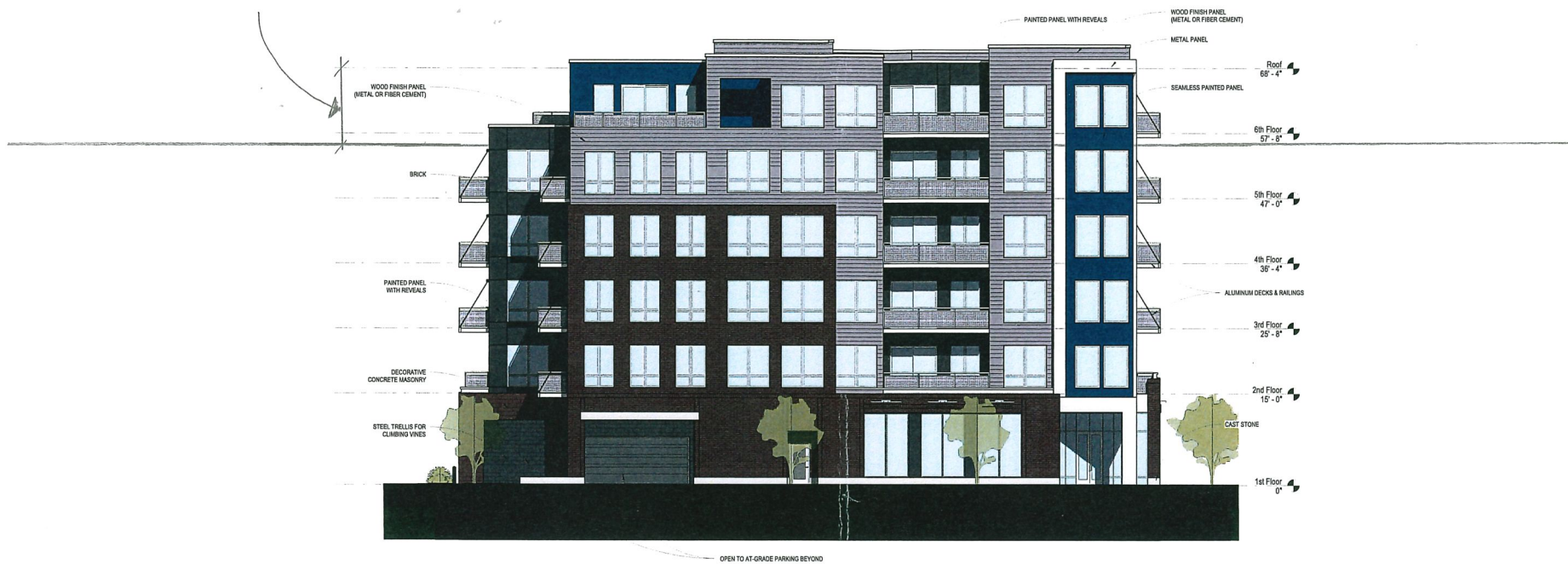
NORTH ELEVATION - ST. CLAIR 1/8" = 1'-0"
