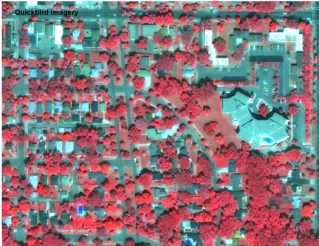
Figure 3. Enlargements of the lidar nDSM (top) and false color (bottom) QuickBird imagery.
