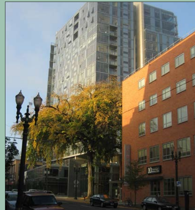
FIGURE 4.4 - These developments in Portland, Oregon define the street with a podium consisting of first-floor retail (top) and density in a smaller point tower above (bottom).
