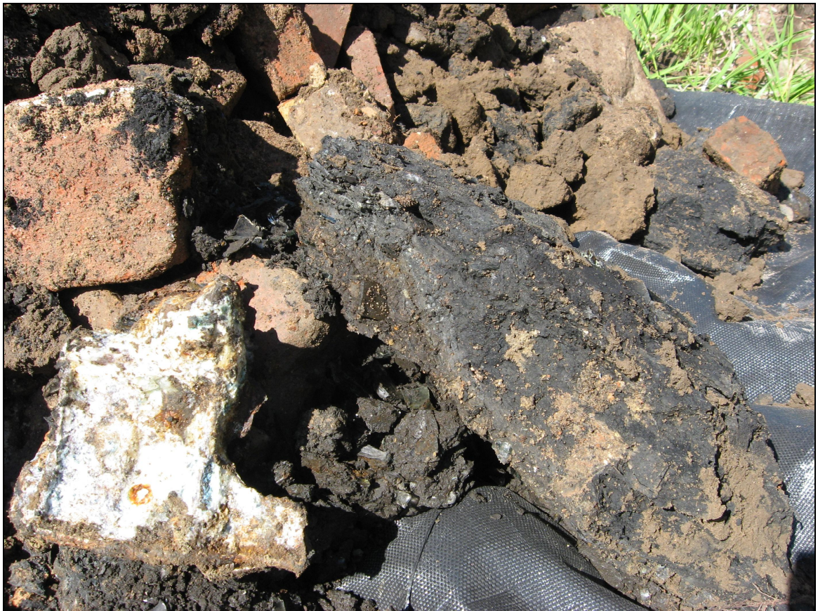
Photograph #4 Subject: Black tarry layer from approximately 12-foot depth in TP-1
