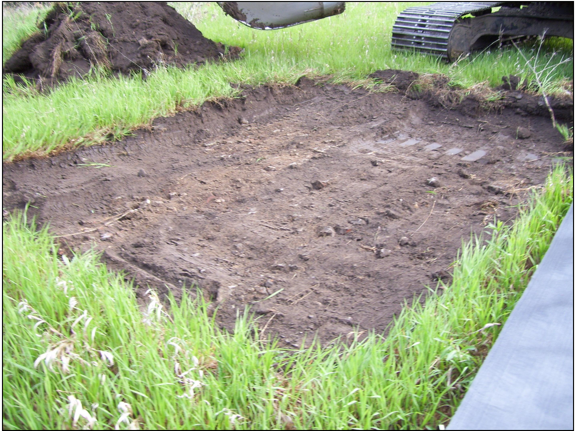
Photograph #1 Subject: Extent of topsoil cover at Test Pit 1 location (fairly typical of all test pits)
