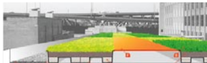
Green roofs can retain up to six times more stormwater than conventional roofing material and provide additional insulation to reduce heat loss.
