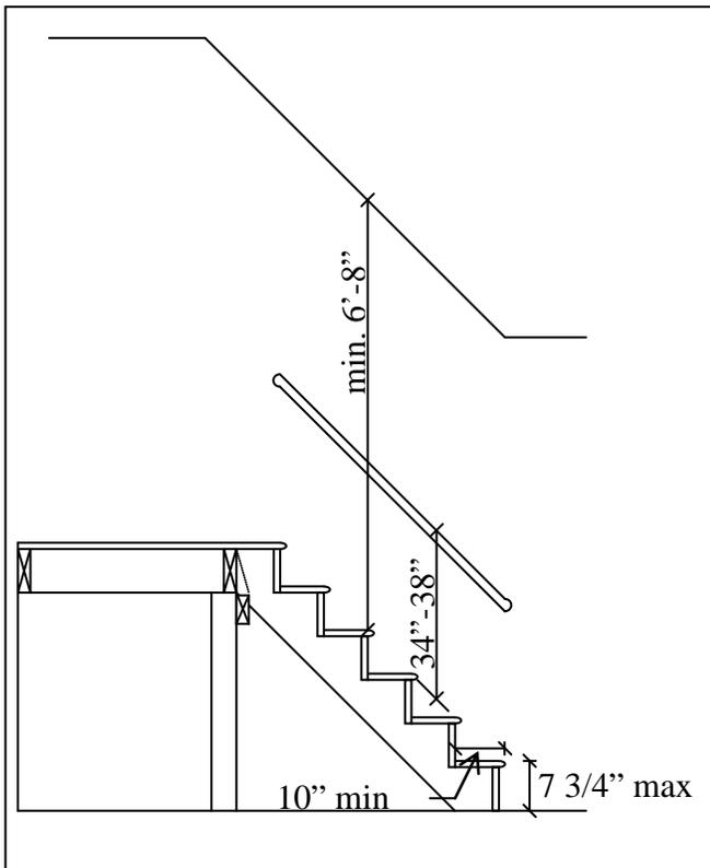
**Width:** Stairways shall not be less than 36" in clear width at all points above the permitted handrail height and below the required headroom height. Handrails shall not project more than 4-1/2" on either side of the stairway and the minimum clear width of the stairway at and below the handrail height, including treads and landings, shall not be less than 31-1/2" where a handrail is installed on one side and 27" where handrails are provided on both sides.
