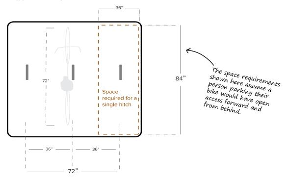
The space requirements shown here assume the area is confined on either side (left and right). Access is located at the top and bottom of the image, requiring a center aisle for circulation.
