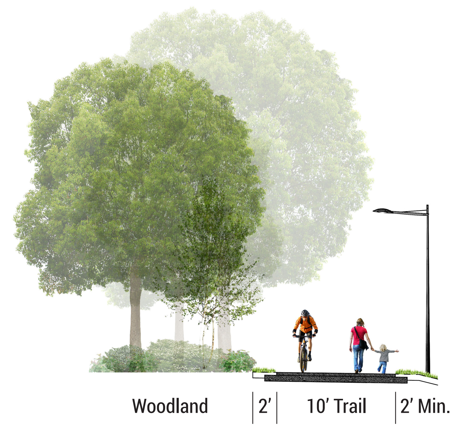
Barge Channel Road - Typ. Section B2
