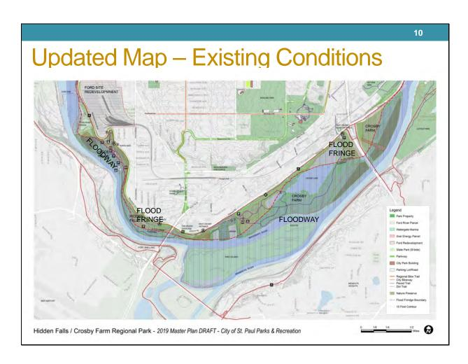
The study of existing conditions builds upon the Great River Passage map and has added more detail representative of what exists at the park. The floodway shows the limit of where structures can be built as it is the zone for flooding. (see presentation PDF for detailed existing conditions map)
