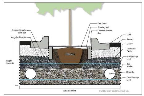
**Figure 5:** *Typical design of tree trench*
