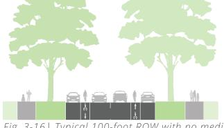
Fig. 3-16 | Typical 100-foot ROW with no median
