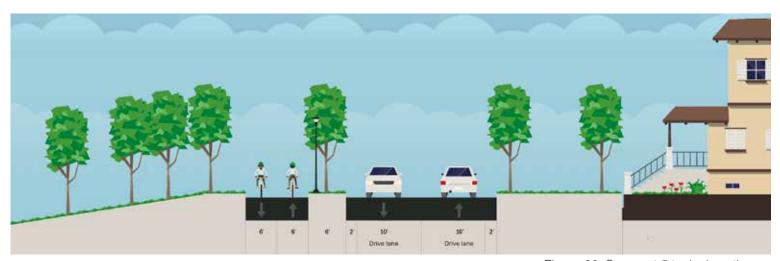
Figure 26: Segment 5 typical section
