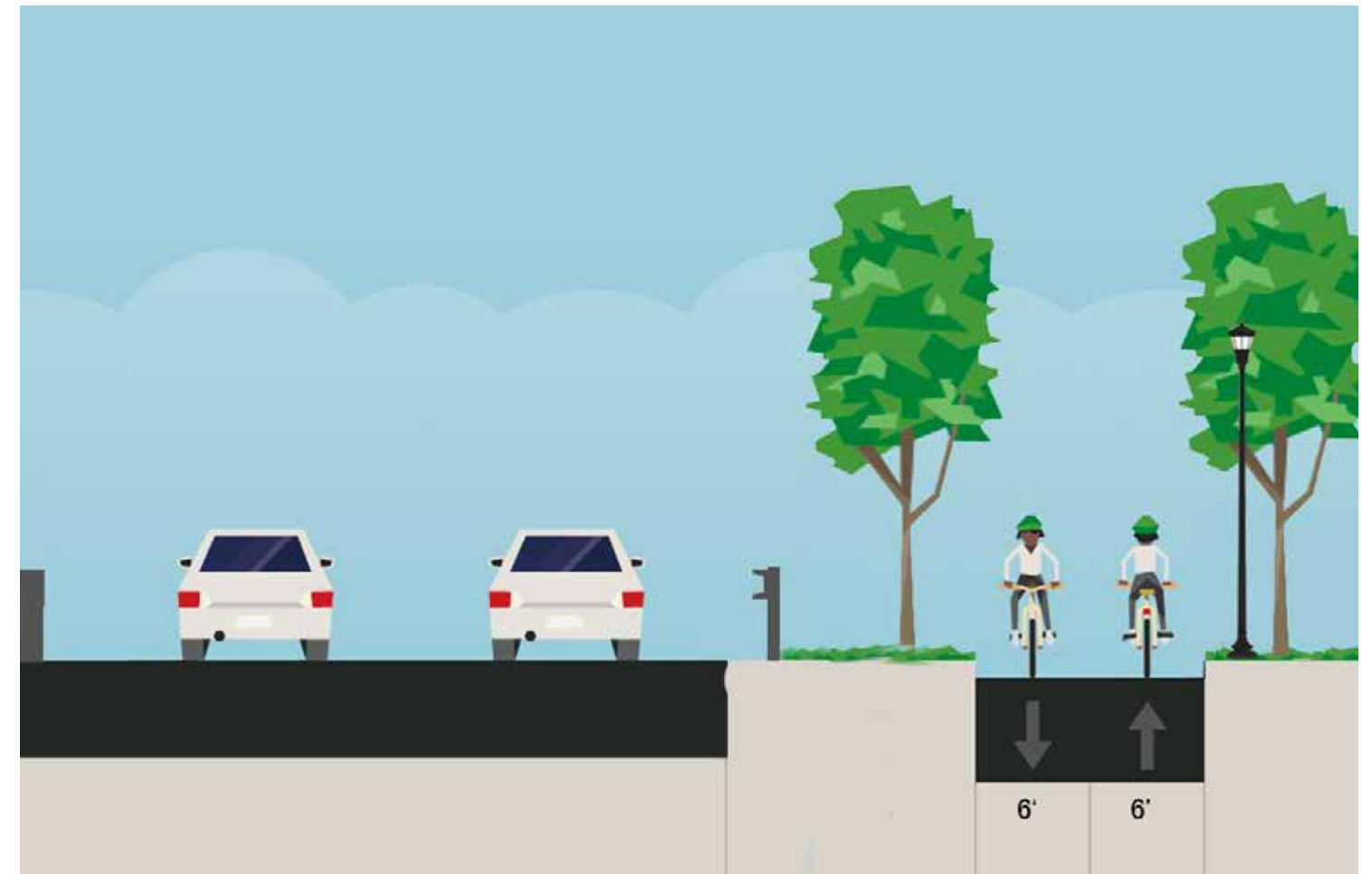
Segment 4 typical section. 12'-0" trail to replace existing 8'-0" trail, new vegetation buffer & pedestrian lights.
